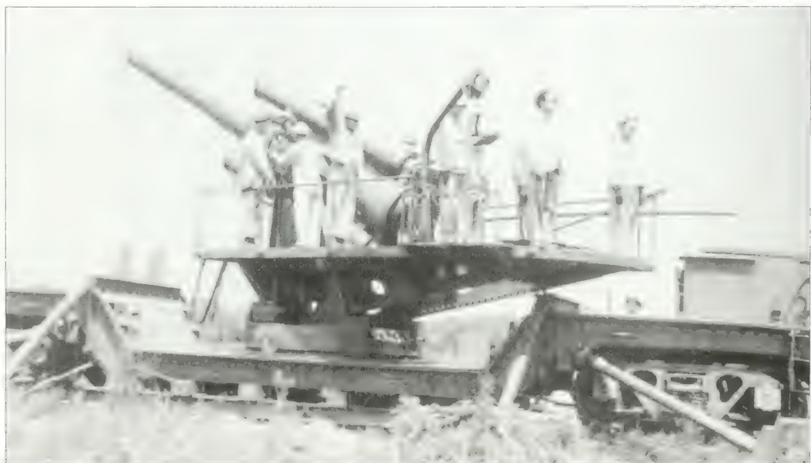
Figure 2.63. 8-inch caliber railway artillery, circa 1939. Mobile artillery was comprised of large caliber guns and mortars mounted on railway cars. The Army positioned two 8-inch caliber railway guns between the dunes facing the shipping channel (Thomas Hoffman, Fort Hancock , Charleston, SC: Arcadia Publishing, 2007).
